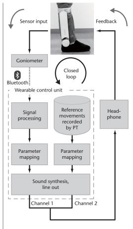
reference using ABF or VBF. For the reference, a physiotherapist (PT) moved one participant's ankle with AFO to record six movement patterns of 60 to 70 seconds. Each pattern comprised a combination of four to seven movements with different speeds. Each movement was about 25 degrees of dorsiflexion and 30 degrees of plantarflexion, taking 6 to 10 s. The dorsiflexion angle was adjusted for some participants because of their limited range of motion.
