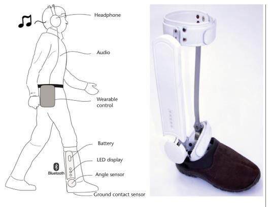
Figure 1. Overview of GaitEcho. The wearable auditory biofeedback device uses an instrumented ankle-foot orthosis for gait rehabilitation.
